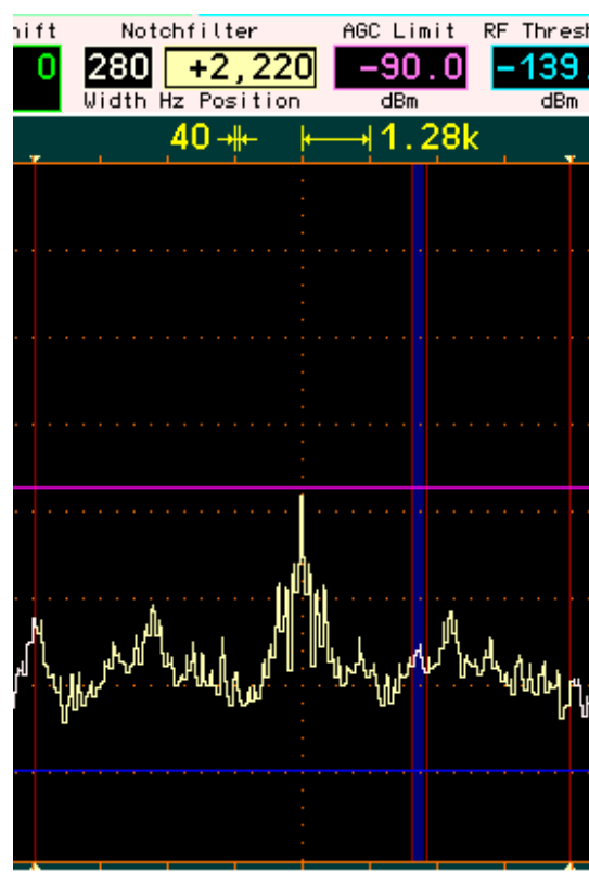
Settings and display of the notch filter.
