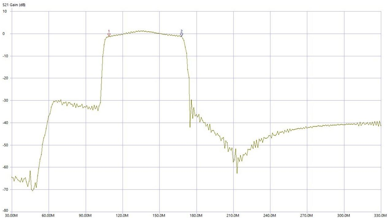
Setting 109 - 169 MHz. A relatively wide filter for digitization mainly in the 2nd Nyquist zone. When selecting a sampling frequency of approx. 180 MHz, alias attenuations of over 40 dB are achieved.
