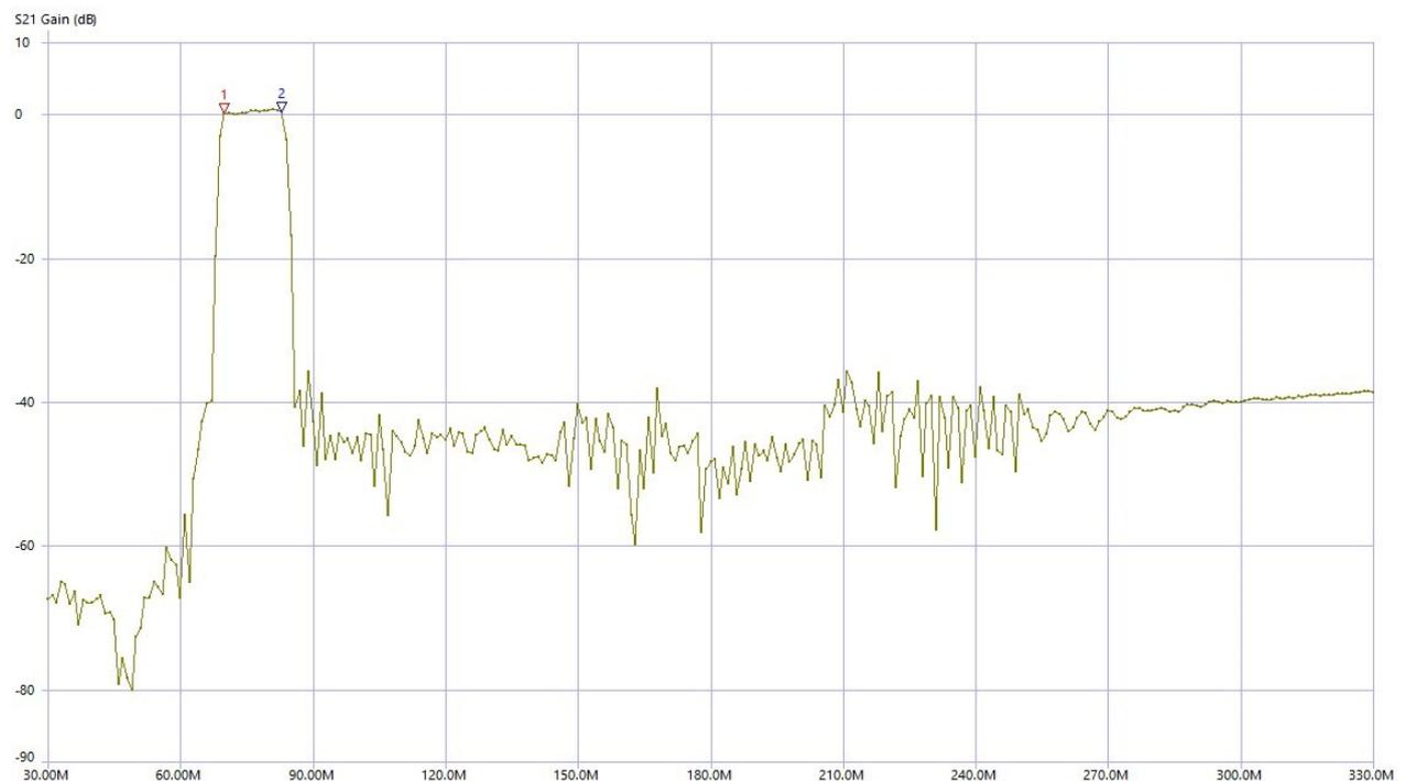
Setting 70 - 83 MHz (marker 1 - marker 2): The filter is optimal for a sampling frequency of approx. 60 - 66 MHz (digitization of the 3rd Nyquist zone). In this case, the alias band below the sampling frequency (2nd zone) is attenuated by more than 60 dB. If the sampling frequency is selected above the passband (2nd zone digitization), over 40 dB can still be achieved.
