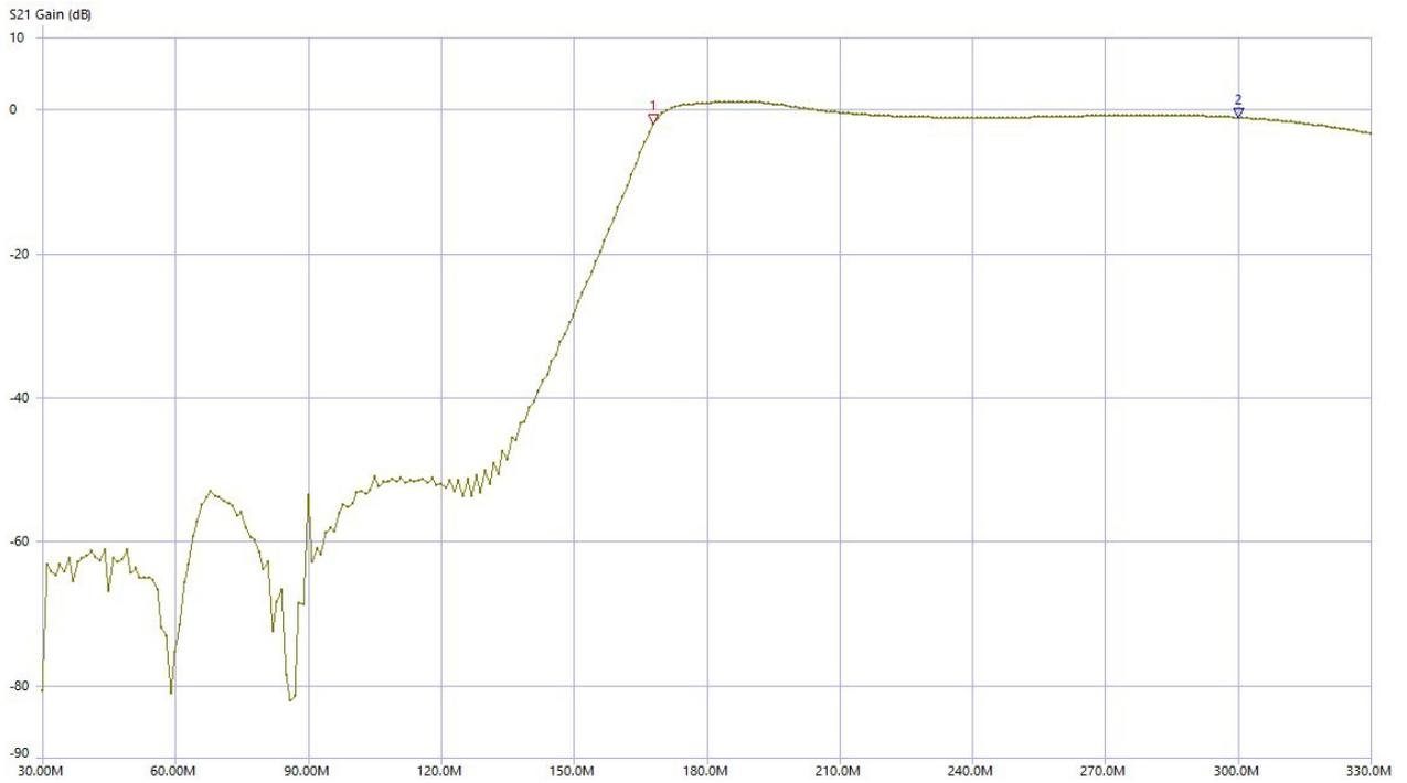
Setting 169 - 300 MHz: Digitization from the 2. Nyquist zone with sampling frequencies from approx. 150 MHz. The high-pass filter primarily suppresses signals from the FM range up to the 2 m amateur radio range. Additional (external) filters are required for alias interference from the higher Nyquist zones.
