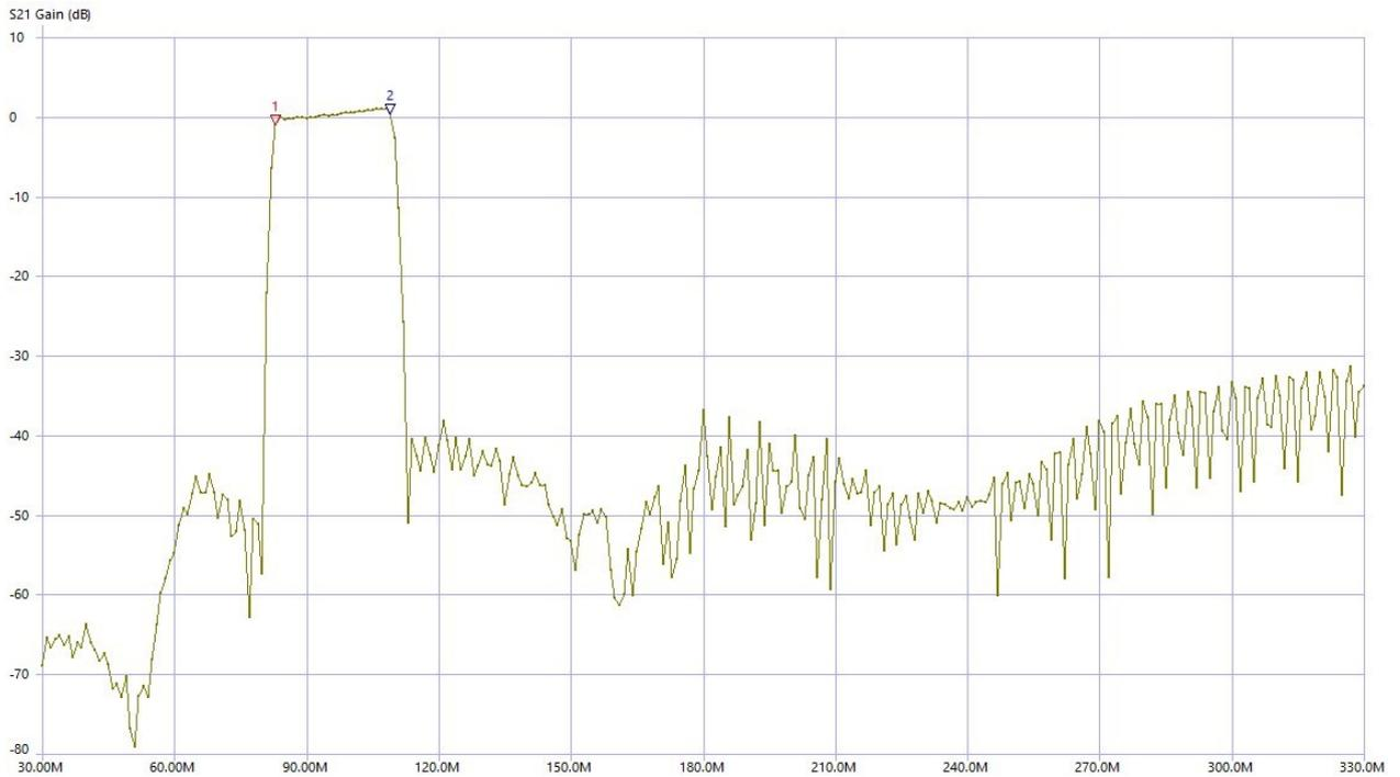
Setting 83 - 109 MHz: Digitization in 2nd or 3rd Nyquist zone. Alias attenuations of approx. 50 - 60 dB can be realized with a suitable selection of the sampling frequency.
