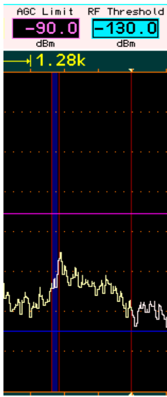
Setting and display of the lowest and highest audible level.
