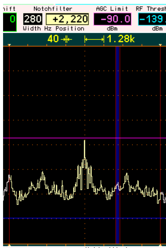
Settings and display of the notch filter.
