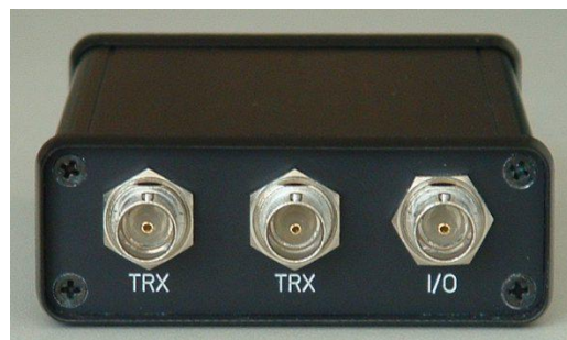
RPP1 passive power splitter / combiner 0.1 - 150 MHz max. 2W:
