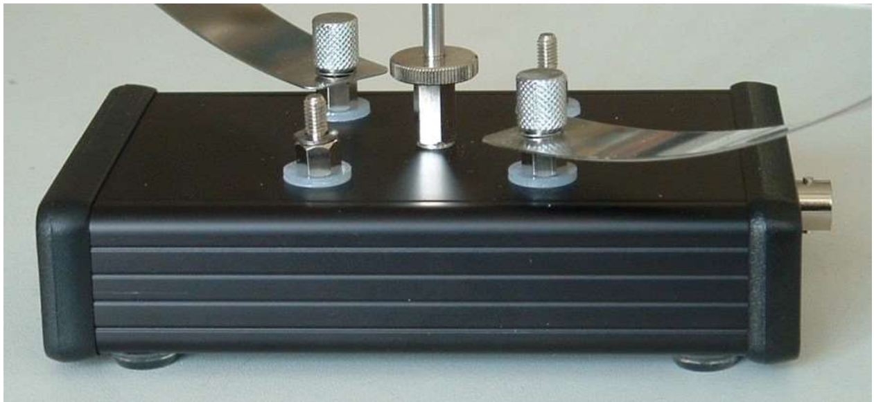
Connection bolt of the amplifier with an installed steel strip
