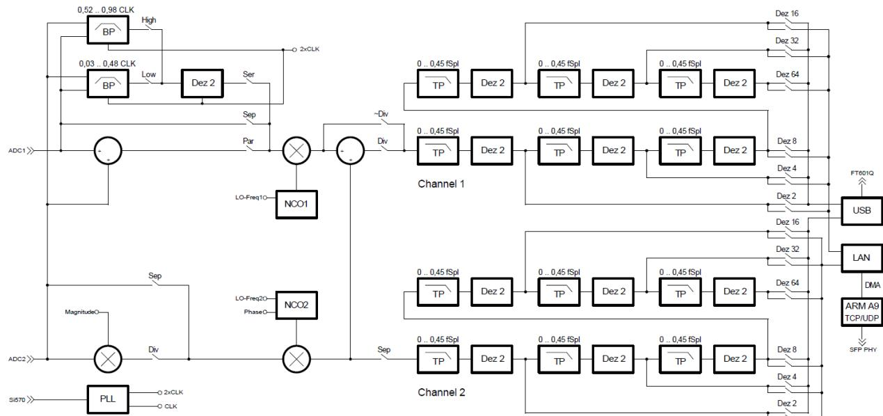
Hardware for digital signal processing inside the FPGA of the RSR200.
