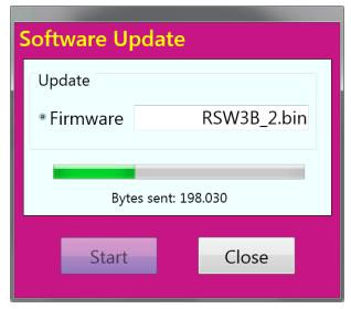
The "Firmware" field is initially empty. With a double click / tap on it, the program searches for transferable files. These files must always have the extension. Bit and be located directly in the ExtIO\*.DLL folder. If there are several \*.Bit files in the folder, the first one that can be found (depending on the arrangement of the files in the folder) is used. To avoid confusion, there should always be only one update file in the folder, namely exactly the (new) firmware to be transferred.
