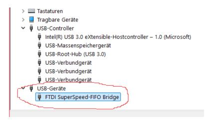
The new "WU" driver can be specified in the Device Manager after opening the properties for the previous FT601 entry under "USB controllers." After updating the driver, only FTD3XXWU.DLL (and the associated ExtIO RSR200B210.DLL) can be used for the SDR program. The old DLLs can be deleted once the new driver is running reliably.
