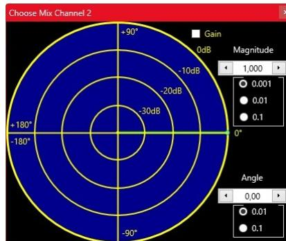
The green pointer can be dragged at the tip (small green dot) with the mouse and dropped in the IQ data space. The distance to the center corresponds to the amplitude (correct: magnitude of the complex signal), the angle to the x-axis corresponds to the phase. If the signal in channel 2 is smaller than that in channel 1, a digital amplification can be switched on via “Gain”. The separately adjustable attenuators in channels 1 and 2 can also be used to influence the signal.
